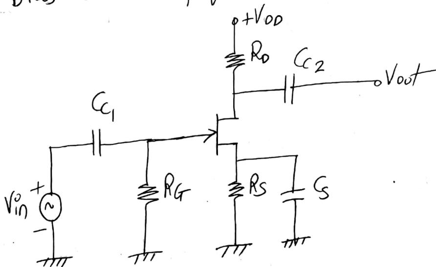
Design means to determine the values of  $R_G, R_D, R_S$
