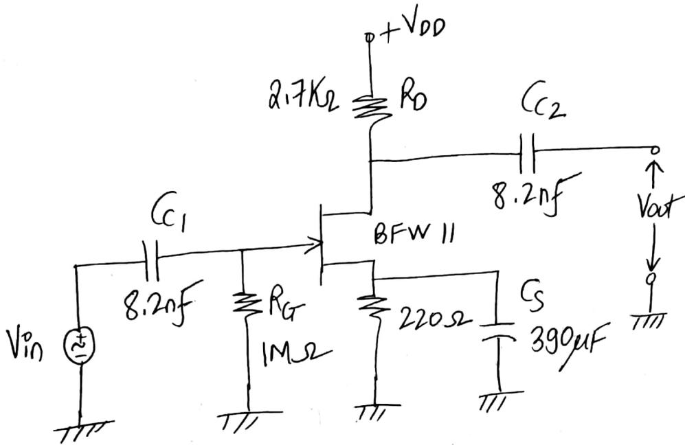
Designed single-stage CS JFET amplifier using mid-point biasing technique
