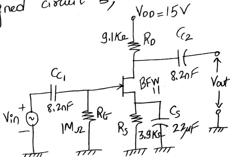
Designed using single stage CS JFET amplifier
