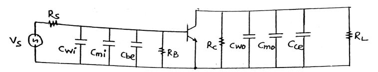
(2) Replacing transistor with model, and input voltage source with current source.
