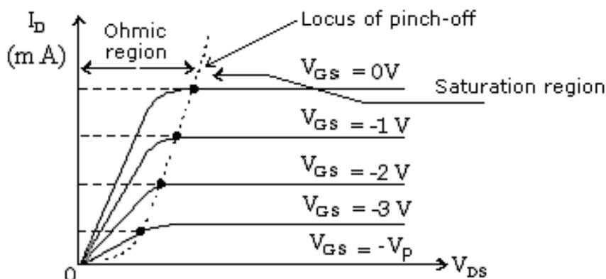
The region to the right of the pinch-off locus is typically employed in linear amplifiers (Amplifier with minimum distortion at applied signal) is commonly referred as the constant current, saturation or linear amplification region.
