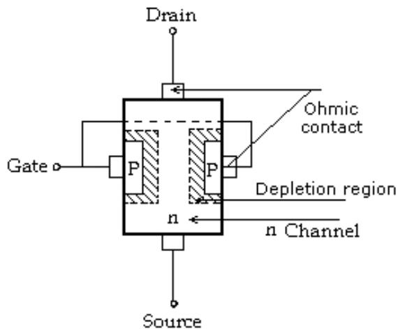
The basic construction of n-channel FET is as shown in figure. The major part of JEET is the channel between embedded P types of material. The top of the n-channel is connected to an ohmic contact called as 'Drain' (D) & lower end of Channel is called as 'Source' (S). The two p types of materials are connected together & to the 'Gate' terminal (G).
