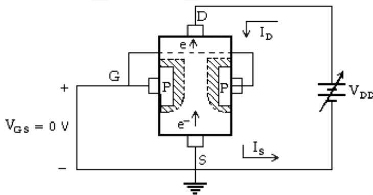
As shown in the figure the gate is directly connected to source to achieve  $V_{GS} = 0V$ , this is similar to no bias condition. The instant the voltage  $V_{DD} (=V_{DS})$  is applied, the electrons will be
