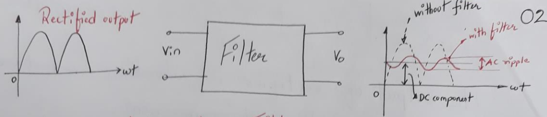
fig: 1.1 Action of a Filter
