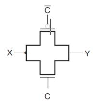
In TG logic design conducting TG network (low impedance path) should always be provided between the output node and one of the inputs, for all possible input combinations. This is to make sure that the output node with its capacitive load is never left in a high impedance state.
