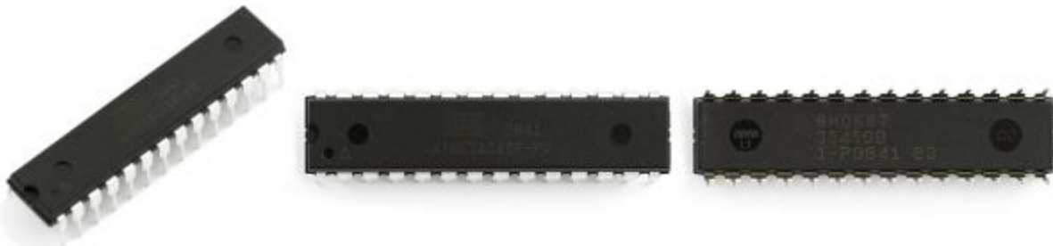
Fig: A 28-pin DIP-packaged microcontrollers
