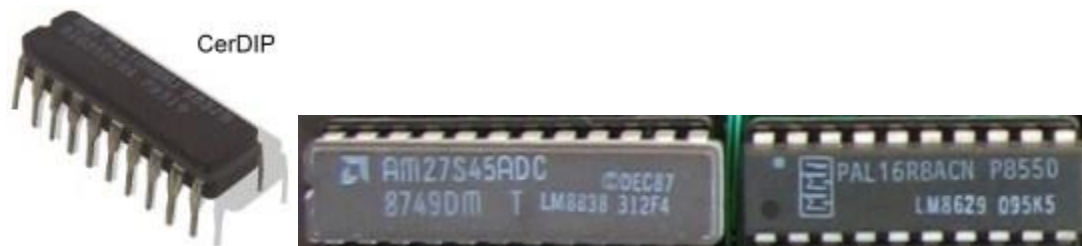
Fig : Ceramic DIP IC
