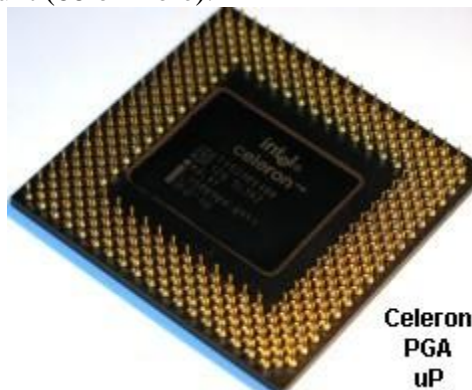
Fig : Celeron PGA Processor
