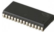
Fig :Photo of a SOJ-28 package, a variant of the SOIC package with J-type leads.
