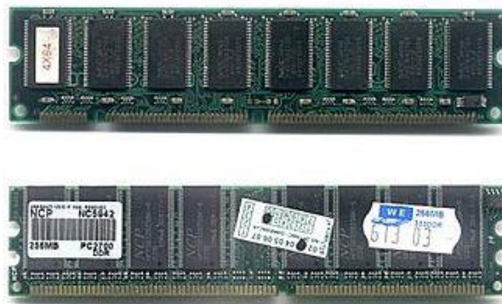
Fig: Two types of DIMMs: a 168-pin SDRAM module (top) and a 184-pin DDR(Double data rate) SDRAM module (bottom). The SDRAM module has two notches (rectangular cuts or incisions) on the bottom edge, while the DDR1 SDRAM module has only one. Also, each module has eight RAM chips, but the lower one has an unoccupied space for the ninth chip.
