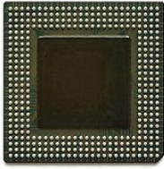
Fig :256 pin perimeter BGA
