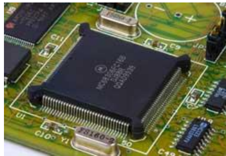
Fig :Bumpered quad flat pack
