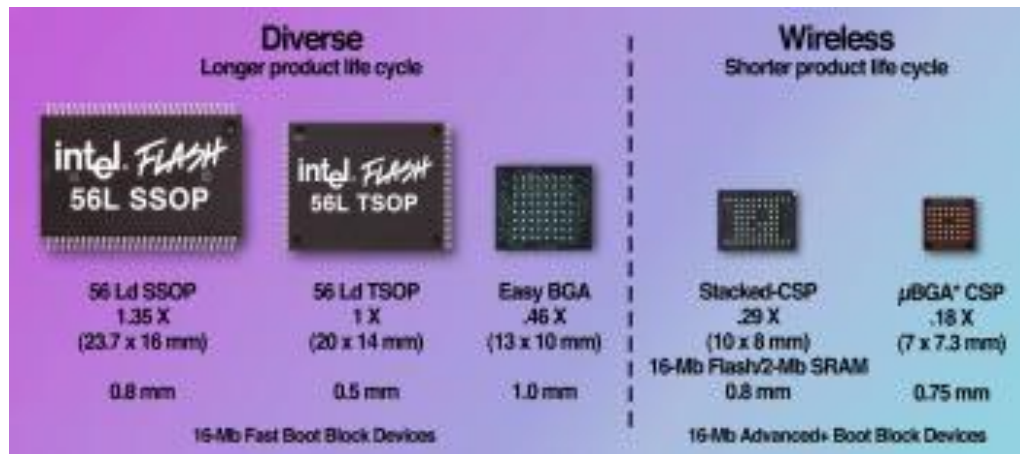
Fig : CSP vs. SOP Size Comparisons
