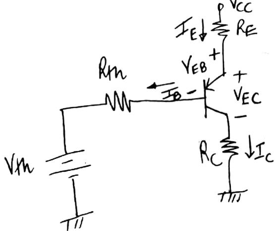
$$V_{th} = \frac{R_2}{R_1 + R_2} V_{cc} = \frac{12k}{3k + 12k} \times 20$$
