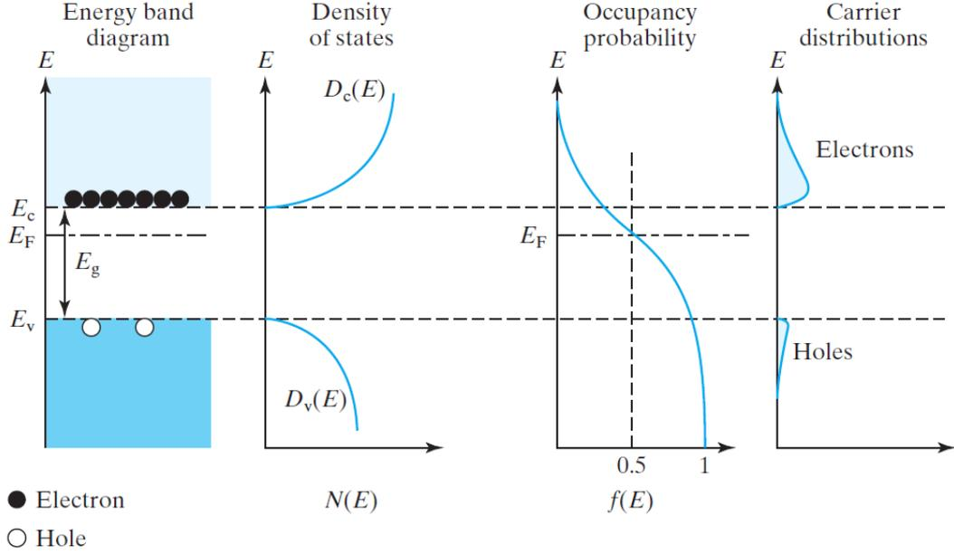
Figure 1: Schematic band diagram, density of states, FermiDirac distribution, and carrier distributions versus energy.
